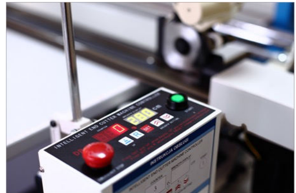
Control panel in Super and Super Plus versions features layer counter, setting the cutting length and the raising height of the cutting track.
